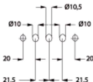
Right- or left-hand handle for use on mechanisms which move the rods that allow closure of the windows with security cylinder. Equipped with a ball mechanism for the positioning of the handle at 90° and 180°.
